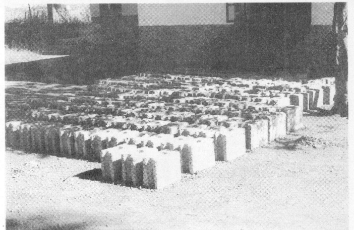
Block production for a tank
